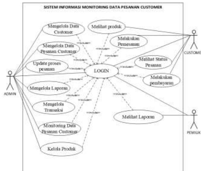
Gambar 2. Perancangan Use case Sistem Monitoring Data Pesanan Customer
